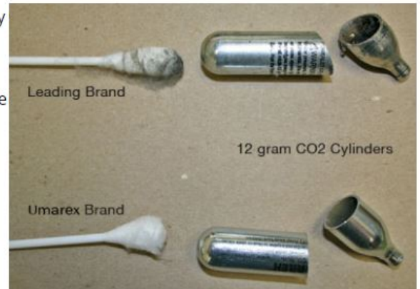
CO2 cartridge cutaway - clean vs. dirty
