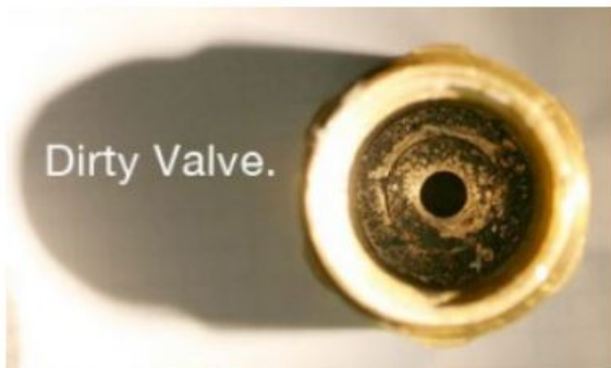
Dirty valve caused by bad CO2
