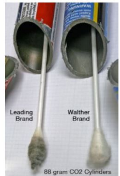
CO2 cartridge cutaway - Umarex/Walther clean vs. dirty brand
